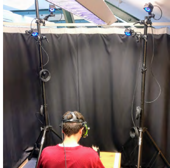
(b) Positioning of the OptiTrack infrared cameras.
