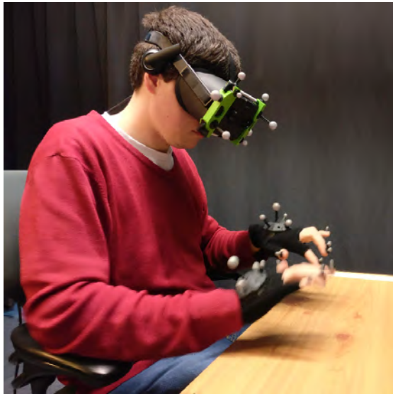
(a) Arrangement of the tracking dots used to track the participant's digits, hands and head.
