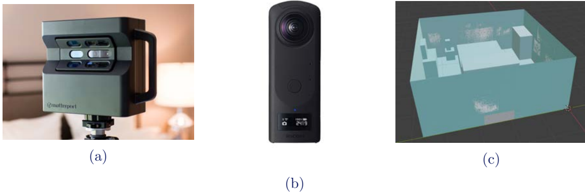
Figure 5: a) Matterport Pro 2 and b) Theta 360. c) We estimate the global transformation for converting points in the sfm coordinate system obtained from images of the Theta 360 to our room coordinates by aligning reconstructed points with primitive objects in our room.
