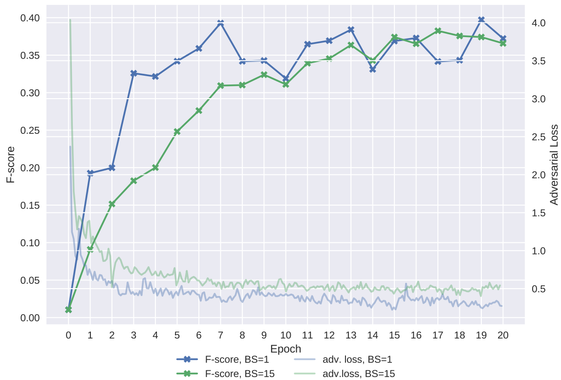
Fig. 5.3 Adversarial training history for different batch sizes. This graph shows F-scores (left scale) on validation data after each epoch of adversarial training, when using batch size of 1 and 15, for the no MLE pre-training. The right scale shows adversarial loss averaged over 1,000 training examples at a time.
