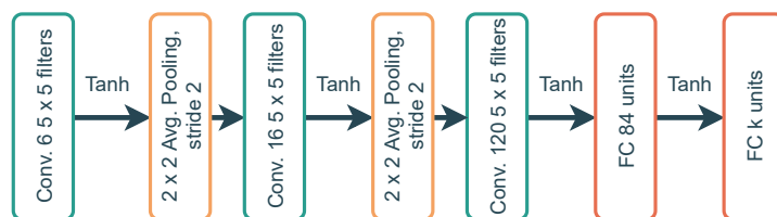
Fig. 3.3 Architecture of LeNet5.
