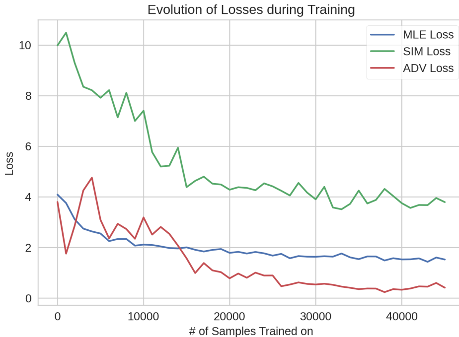
Fig. 5.14 Evolution of the different losses during training, averaged every 1000 samples and using the combined loss with \alpha=0.3 , \beta=0.2 .
