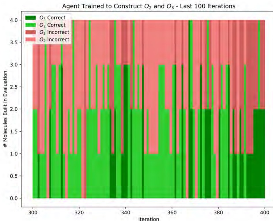
Fig. 4.1 An agent is trained to construct both O_2 and O_3 through randomized penalties. We classify the molecules built over 4 evaluation rollouts for each of the final 100 training iterations. Evidently, the agent learns to always construct either O_2 or O_3 but often chooses the incorrect molecule to build. O_3 Incorrect means that the agent built O_3 when the oxygen penalty increased after 2 oxygens were placed and thus could've achieved a higher reward by building O_2 . Similarly, O_2 Incorrect means that the agent built O_3 when the oxygen penalty did not increase after 2 oxygens were placed and thus could've achieved a higher reward by building O_3 .
