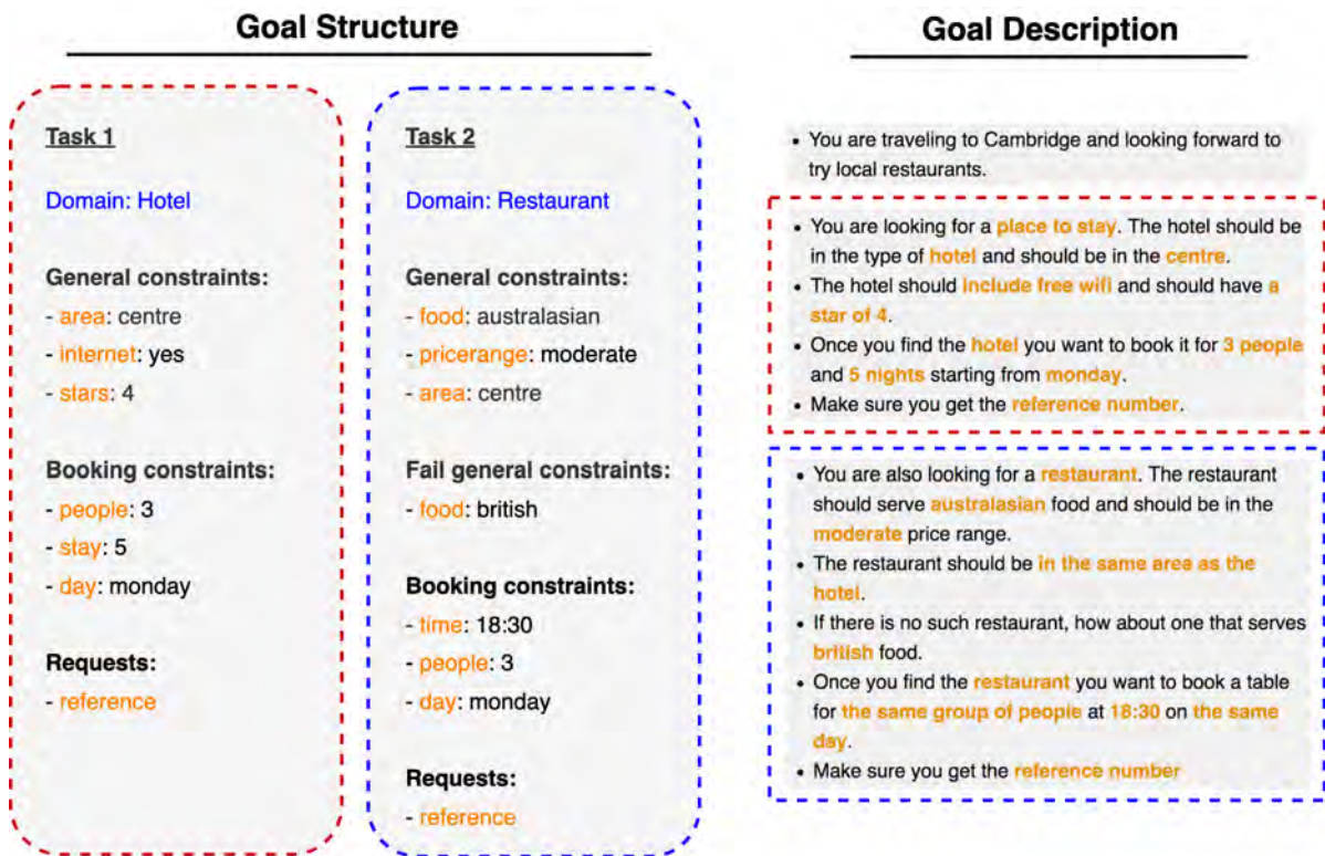
Fig. 2.9 Visual example of a MultiWOZ goal model presented alongside the goal description that was used in the annotation process when the dataset was created. The goal descriptions are from Budzianowski et al. (2018).
