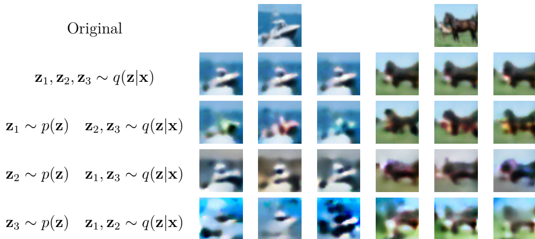
Fig. 3.4 Example reconstructions from a hierarchical VAE. Top row are the original images and the second row are normal reconstructions. For each row after that, one of the latent variables is sampled from the prior. It shows each latent variable learns different features that control different aspects of the reconstructions.
