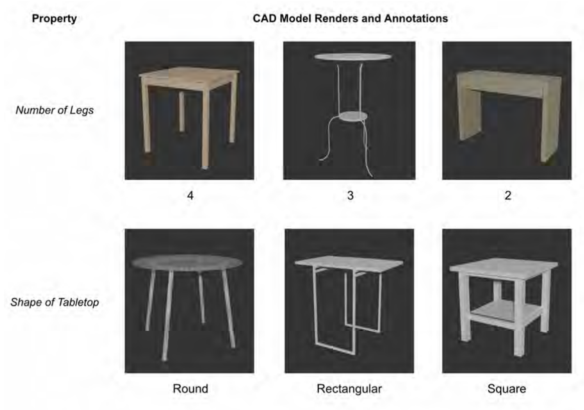
Fig. 3.2 Examples of table properties and annotations. Properties are in the left column and each annotation for the property is below its corresponding table image. Each property provides key information that can help our system filter through a database of different CAD models.
