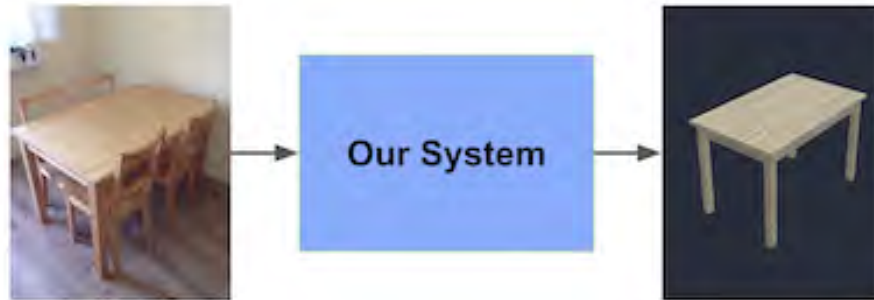
Fig. 1.1 Our system takes in an image of an object as input. We output a CAD model, rotation matrix, and translation vector where the CAD model is aligned with the image when placed at the outputted rotation and translation, as visualized in the render on the right.
