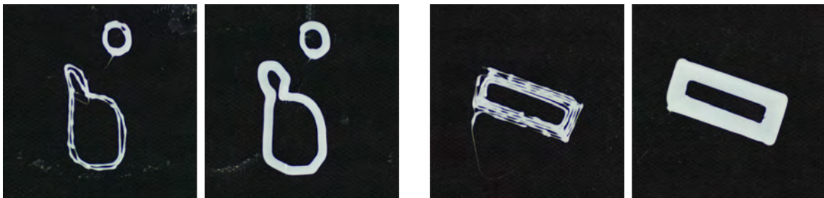
Figure 1.2: The Effect of Different Process Parameters. The same input geometries printed with different flow rates.
