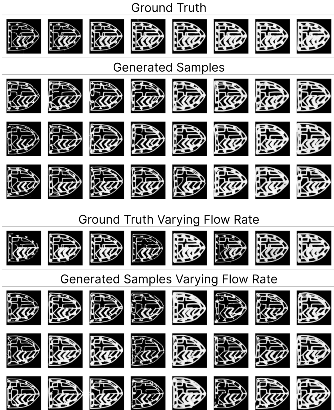
Figure 4.15: Clare College Crest Data and Generated Samples. This figure presents printed layer images of the Clare College crest, and generated samples from the same input graph underneath. The top half use linearly spaced but constant flow rate. The bottom half have randomly varying flow rates.
