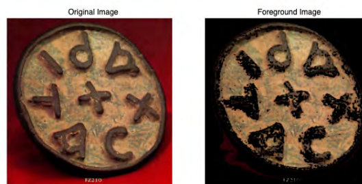
Fig. 6.1 Original image (left) and foreground image (right) after background subtraction applied.
