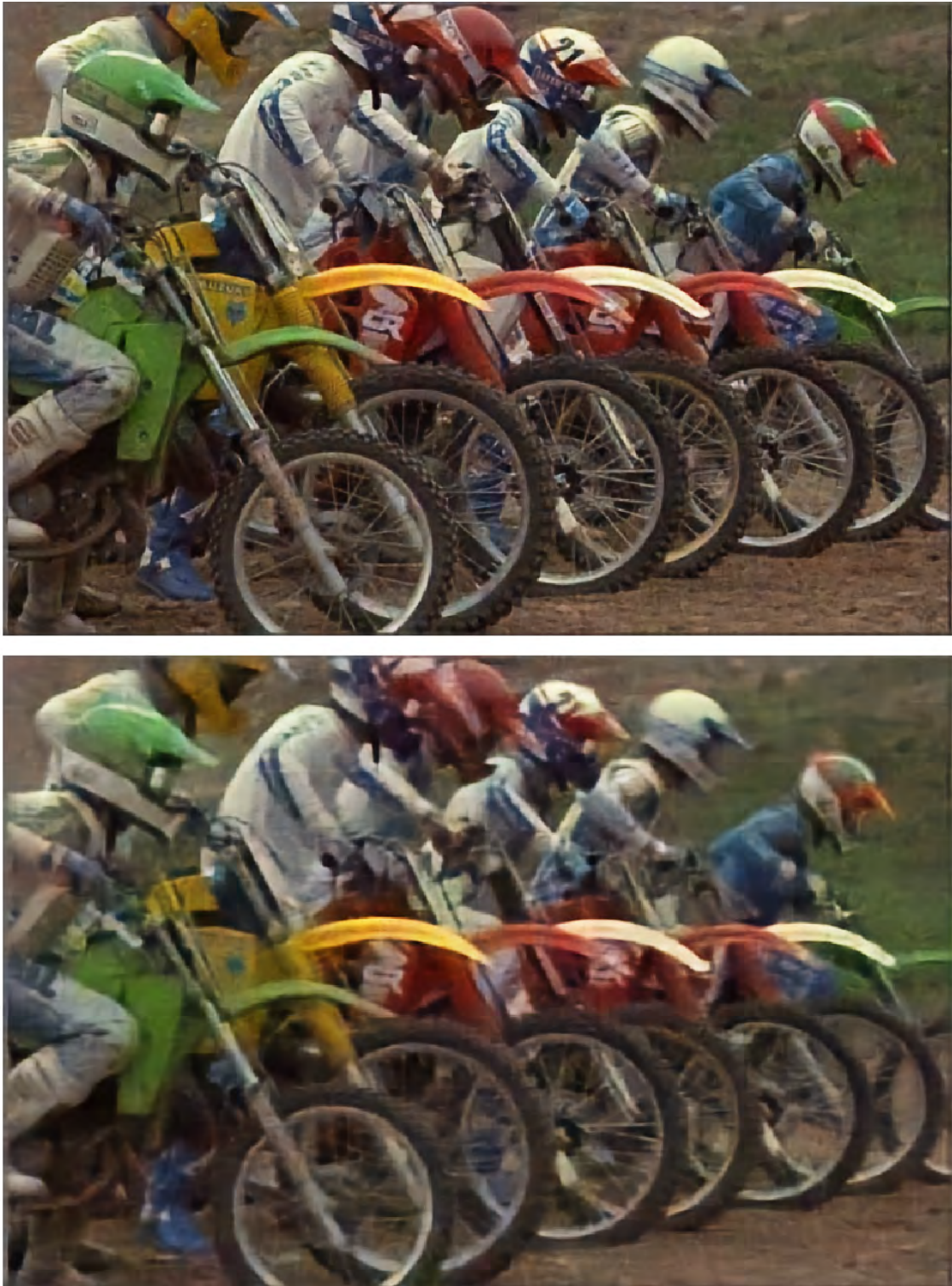
Fig. 5.2 \gamma -PLN reconstructions of kodim05. Top: \beta = 3 , 0.354 bpp, MS-SSIM: 0.937, PSNR: 21.397 dB Bottom: \beta = 10 , 0.189 bpp, MS-SSIM: 0.824, PSNR: 21.068 dB.
