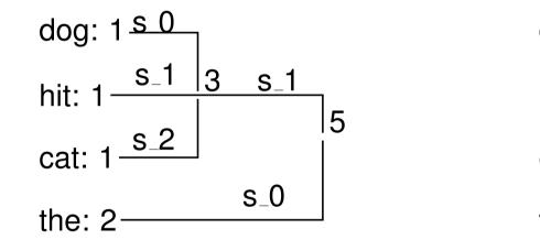
Figure 3: Example of the Huffman coding scheme
