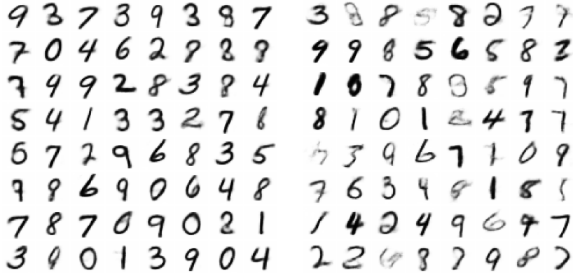
Fig. 2.6 Left: Digits generated from the inner latent space of a two-level VAE trained on MNIST. Right: Digits generated from the latent space of a VAE trained on MNIST. \mathbf{u} and \mathbf{z} are drawn from \mathcal{N}(\mathbf{0}, I) .
